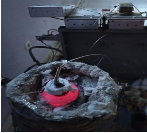
Gambar 3 Proses Peleburan 86 Al 1020 – 12 Fly ash – 2 Mg
